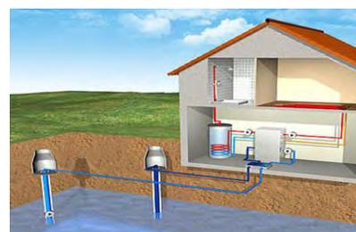
A low-enthalpy geothermal open-loop system
