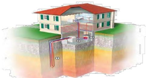
A low-enthalpy geothermal closed-loop system
